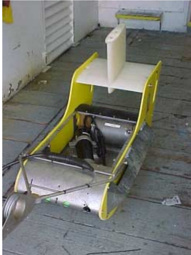
Figure 9. Chelsea Systems undulating towbody. An Applied Microsystems Ltd. Sound Velocity SVP-16 velocity profiler is bolted in place.
