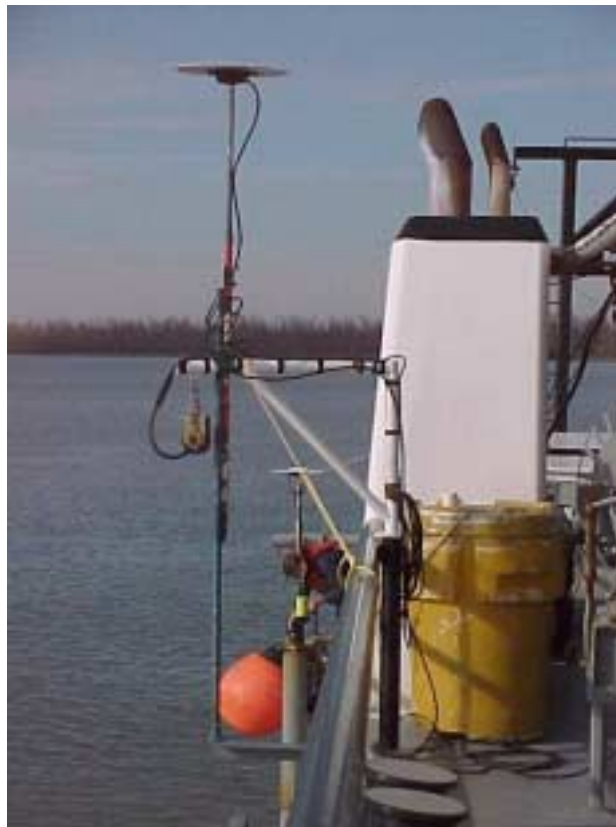
Figure 8. Static Calibration of real-time draft sensor. GPS Antennas mounted for OTF Kinematic tests.
