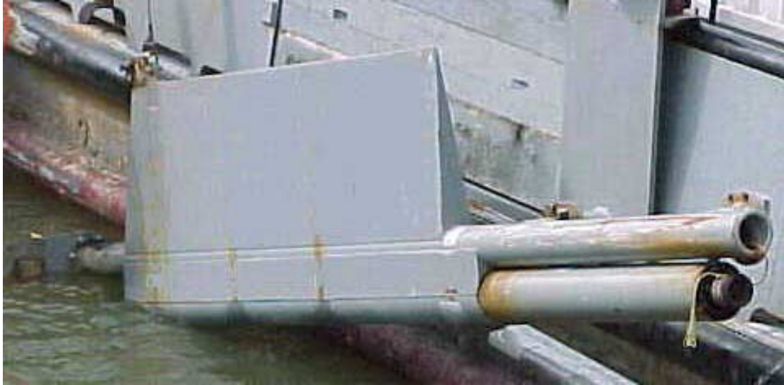
Figure 4. Ram being lowered for testing. The top pipe is the multibeam transducer pipe with vertical beam transducer mount; the bottom pipe is the draft sensor pipe. Also shown is the stabilization fin.
