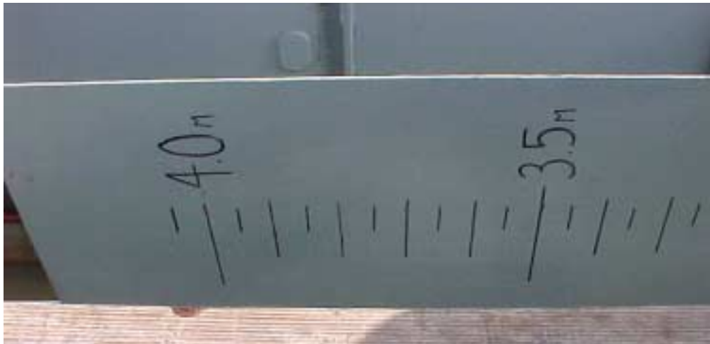
Figure 6. Draft markings on stabilization fin of transducer pole.
