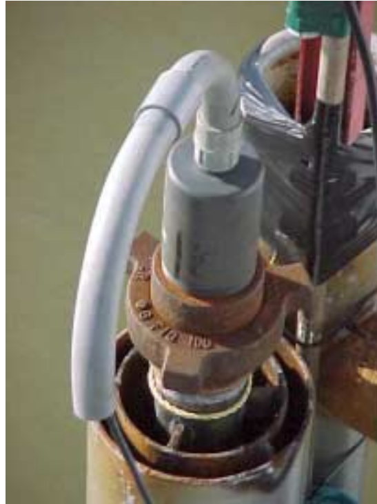
Figure 7 Draft sensor showing multipipe system.
