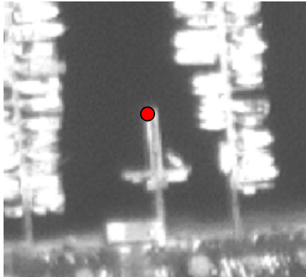
Figure 3A. Image location of a GPS point used in the image georeferencing process.
