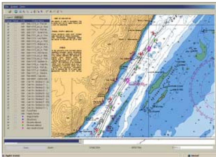
Figure 5. An example in the St. Lawrence River combining BSB Raster Nautical Chart overlain by channel vector information, the National NavAids database and the Regional Shoals Database viewed in this seamless environment and distributed over the Internet with CARIS BEAMS. All data courtesy of the Canadian Coast Guard.
