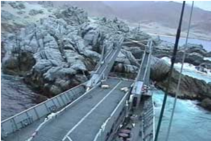
Figure 1. USS LA MOURE COUNTY aground in Caleta Cifuncho Bay, Chile after navigating with GPS (WGS-84 datum) on a local chart on local datum. The Navy has decided to write off the 29-year-old, 561-foot vessel and sink it.
