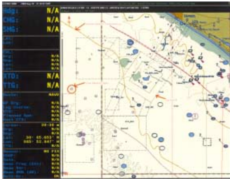
Figure 4. Static AMLs overlain on a Field DNC® of Panama City, FL displayed on Offshore Systems Ltd. (OSL) ECPINS. Shown are operational areas, bottom targets, and sediment contours.
