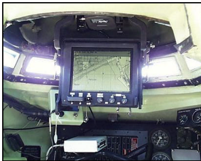
Figure 6. View from inside the AAV showing the driver's station with NRL-MM display and windows to outside view.
