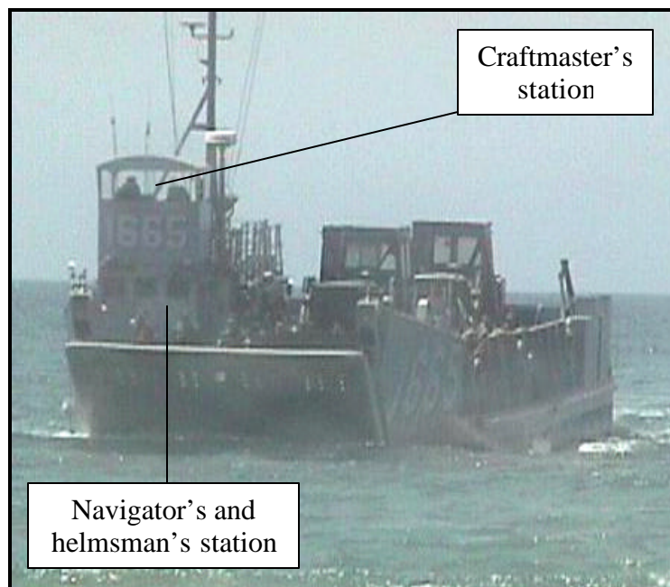
Figure 1. A Landing Craft Utility (LCU) showing primary crew locations.
