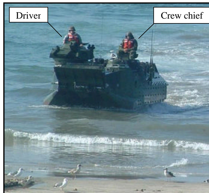
Figure 2. An AAV coming onto the beach (note: crew chief and driver are often partially or completely inside vehicle; communications are hampered by surf and engine noise).
