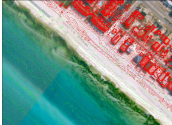
Figure 2. Imagery with topographic and hydrographic lidar survey of the coastal zone.
