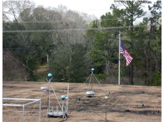
Figure 5 – Two C-Nav units (front row) on the roof of an adjacent building.
