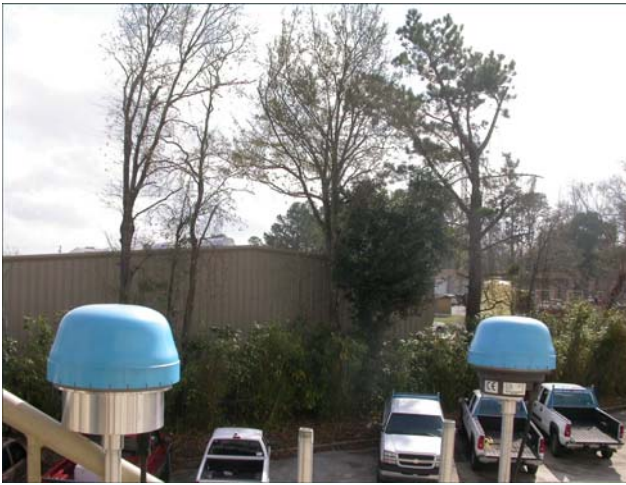
Figure 3 - South view of two C-Nav units in a high blockage and multipath environment.
