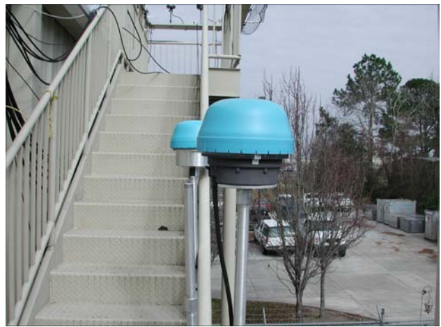
Figure 2 - West view of two C-Nav units in a high blockage and multipath environment.
