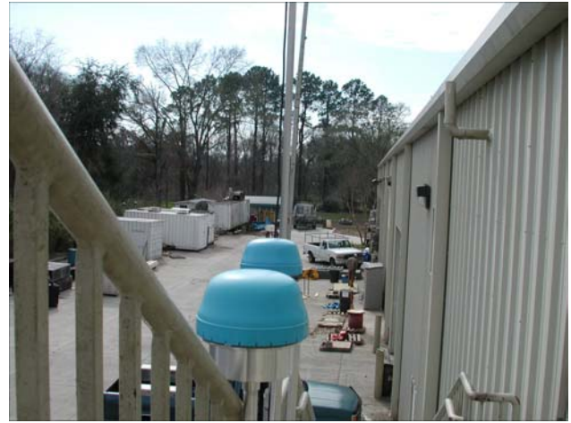
Figure 4 - West view of two C-Nav units in a high blockage and multipath environment.
