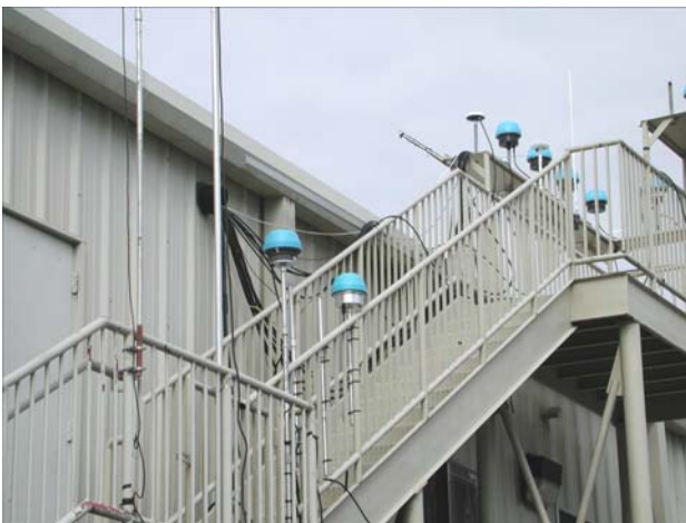
Figure 1 – Northeast view of two C-Nav2000 units (to the left) in a high blockage and multipath environment.
