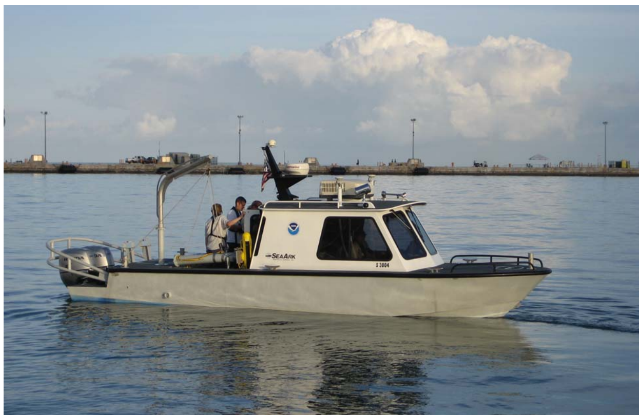
Figure 2 – The NRT-7 vessel, S3004, is a 29' aluminum hulled SeaArk and is equipped with state of the art hydrographic survey equipment. Note the pole mounted C3D phase differencing sonar.
