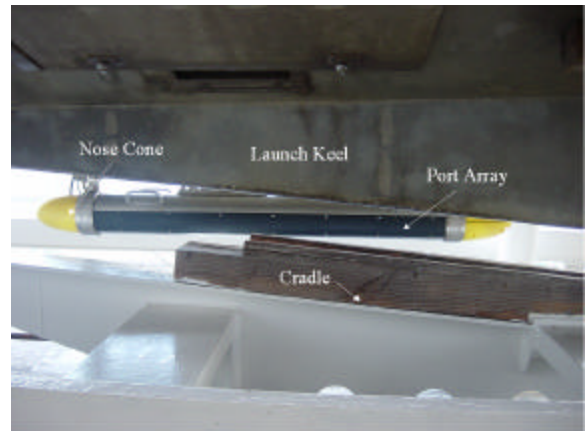
Figure 2: Photograph of the clearance observed between the top of the port Klein 5410 transducer and the bottom of the launch's keel.
