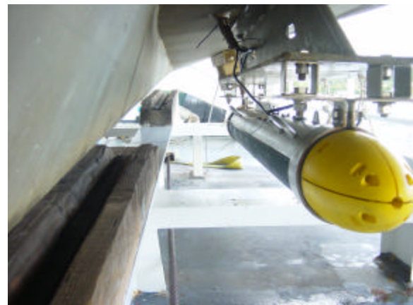
Figure 3: Photograph of the mounted Klein 5410 towfish from the aft end of the survey vessel. The vertical grooves in the tail cone and omega bracket were used as visual references to remove as much of the roll bias as possible.
