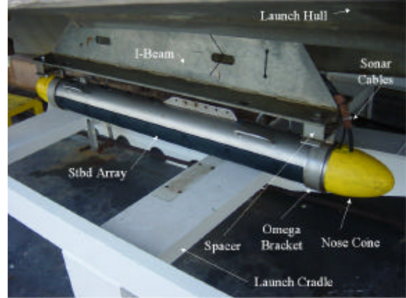
Figure 1: Photograph of the Klein 5410 towfish installed in the Series 5000 mount aboard NOAA Launch 3102.
