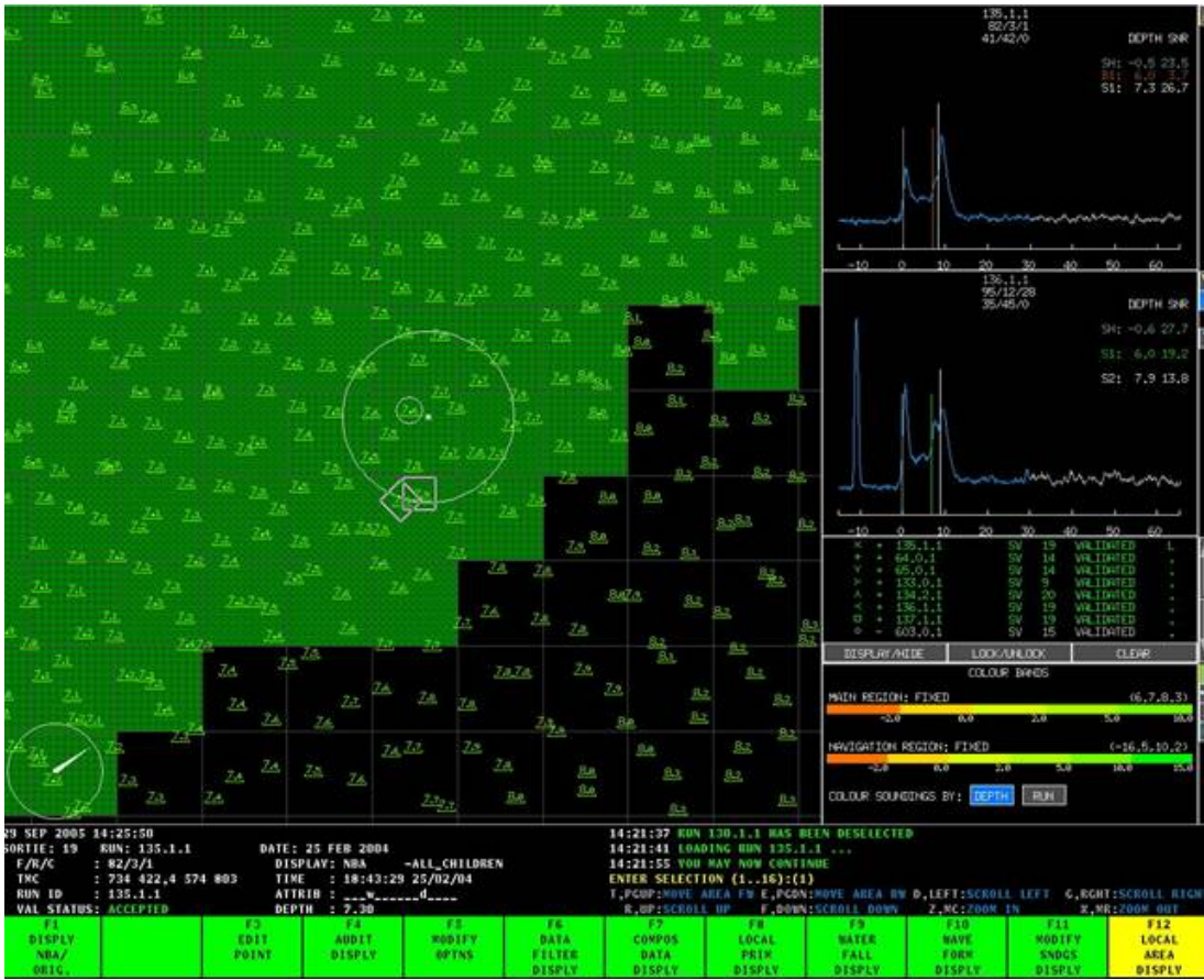
Figure 4 – Automatic algorithms successfully detecting object subsequently removed in manual cleaning. Local Area Display showing selected waveforms (with manual edits) and all surrounding depths.
